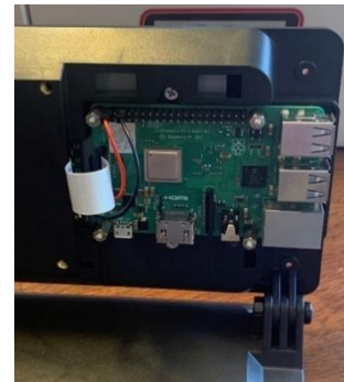
FIGURE 5: RASPBERRY PI 4B MOUNTED TO TOUCH SCREEN DISPLAY
